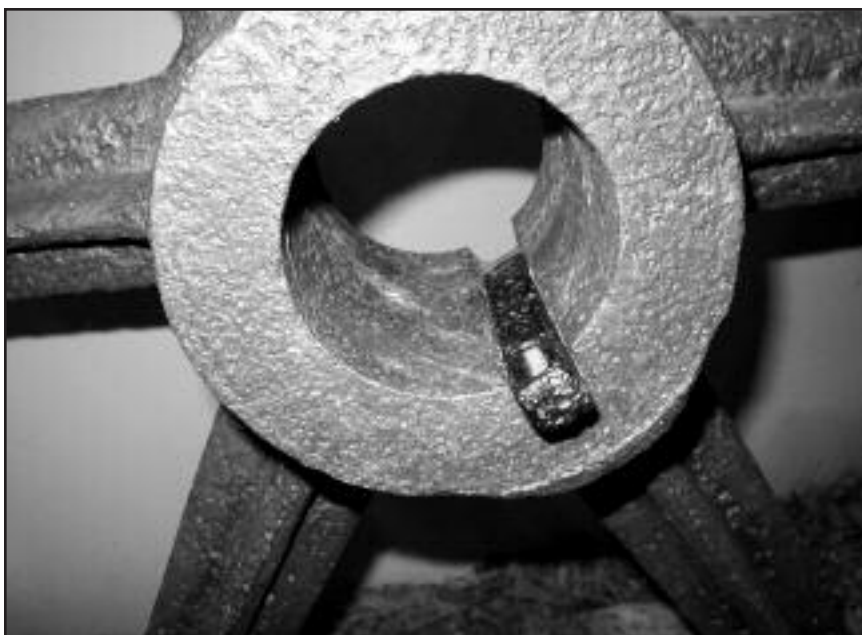
Haun's Mill face wheel shown with the locking or wedge pin in the inside groove, LDS Museum of Church History and Art, Salt Lake City, Utah, 14 November 2003. Photograph by Alexander L. Baugh.
